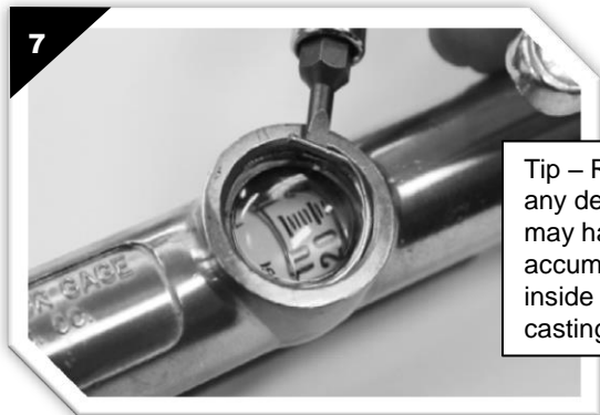
STEP #7 – Use small blade screwdriver or small pick to pry retaining ring from inside viewing window cavity
