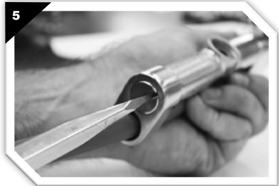
STEP #5 – Remove nut with large blade screwdriver by turning counter-clockwise
