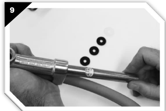
STEP #9 – Insert new cartridge into casting with numbers facing toward handle
