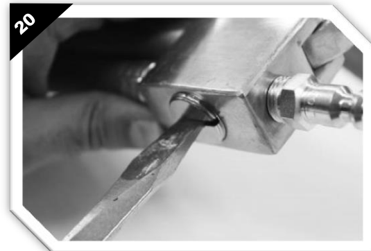
STEP #20 – Replace nut and turn clockwise with large bladed screwdriver to tighten
