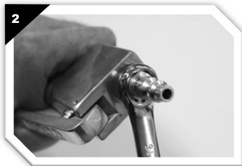
STEP #2 – Remove plug from end of inflator gage
