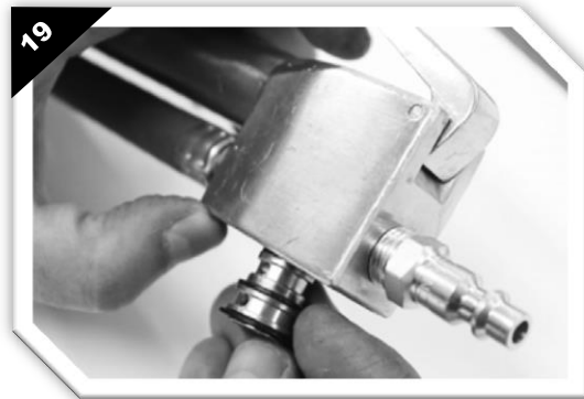
STEP #19 – Insert new valve by pushing in all the way
