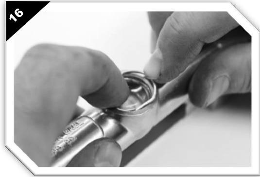
STEP #16 – Insert new plastic viewing window and snap retaining ring into groove to hold viewing window in place
