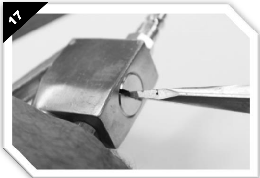
STEP #17 – Remove valve nut with large flat blade screwdriver and turn counter-clockwise
