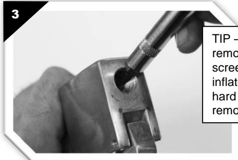
STEP #3 – Remove old inlet screen by prying out with small blade screwdriver
