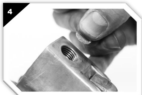
STEP #4 – Insert new inlet screen and gently seat into place with small blade screwdriver
